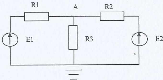
$R1=400 \Omega$ ,  $R2= 200 \Omega$ ,  $R3= 1200\Omega$ ,  $E1= 6$  Volts,  $E2=12$  Volts
