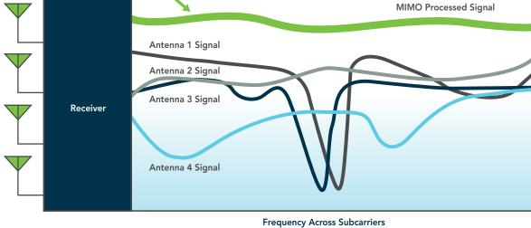
Multiple-in multiple-out (MIMO) signal processing uses multiple antennas, taking advantage of multipath reflections to improve signal
